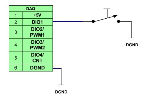
\*All ground wires in the drawing must be connected or no loop can be formed
